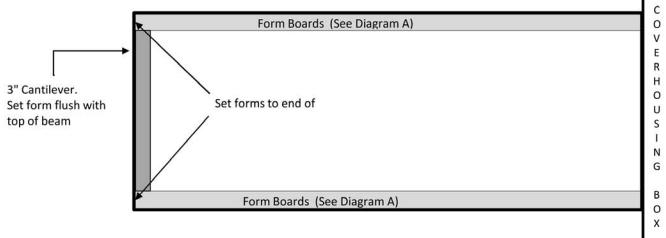
Arizona Pool Covers will insert a Styrofoam insert into the 1.5 inch x 3 inch opening of the pre installed form boards.
