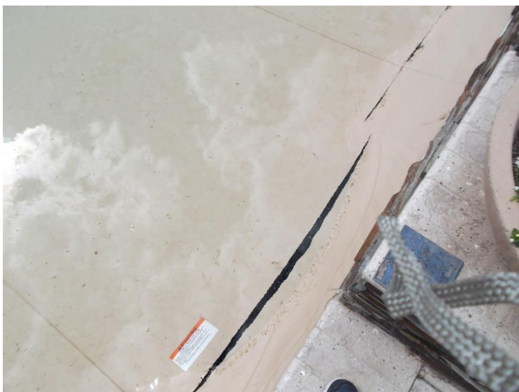
Example of fabric torn from rubbing on Extended Vanishing Lid bracket
