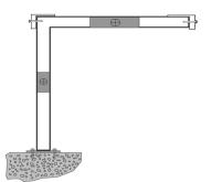
Three-piece adjustable steel brackets provide a maximum height of 20" by 24" wide. Surface material is not included, or installed by
