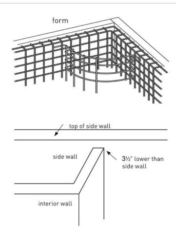
Any interior wall, such as for spas, also must be gunited 3½" (3" finished with tile) lower than the side walls.
