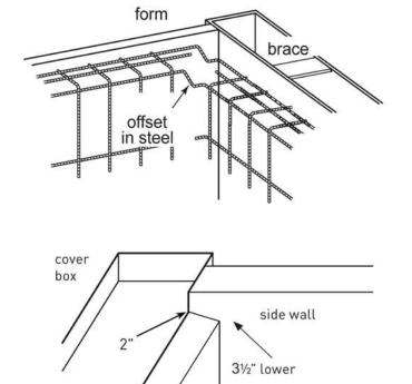
At the recessed box end, the pool wall (bond beam) must be shot 2" ( $1\frac{1}{2}$ " finished with tile) lower than the side walls. And  $3\frac{1}{2}$ " on pool side.
