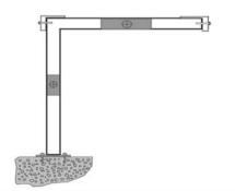
Three-piece adjustable steel brackets provide a maximum height of 20" by 24" wide. Surface material is not included, or installed by Arizona Pool Covers.
